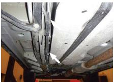
At the front of the fuel tank, find the hard fuel and brake lines. Route the 4-flat along these lines to the rear of the front wheel. Once you have reached the front wheel, route the 4-flat between the vehicle body and the front suspension mount.
