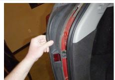
Remove the two Phillips head screws securing the taillight to the vehicle. Carefully remove the taillight by pulling straight back.
