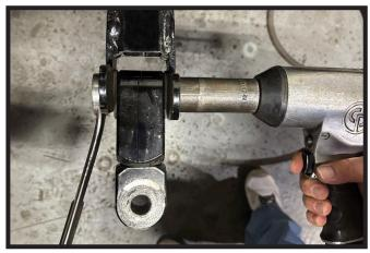
Using a 1-1/8" socket and wrench, remove the one (1) bolt attaching the pivot block to the receiver. Remove bolt and washer, set aside to be reinstalled. Discard old pivot block.
