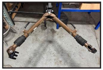
15. Once all the bolts have been fully tightened the tow bar should be able to sit vertically with legs extended as shown.
