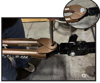
3. Using the alignment tool, align all of the holes on the tow bar. Insert 3/4" x 3-1/2" bolt through aligned holes (inset).
