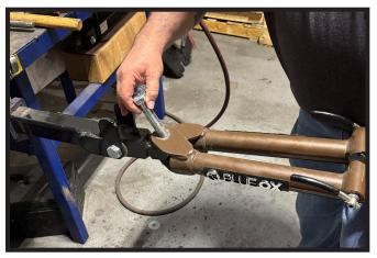
Rotate tow bar out of stowed position. Remove the 3/4" x 3-1/2" bolt. Remove tow bar legs and set aside to be reinstalled later.
