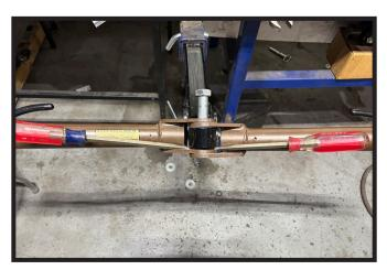
10. Insert the flat screwdrivers into the space that does not contain a washer. Tap on the end of the screwdrivers with rubber mallet to create a gap for the washers to be inserted.
