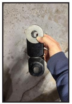
4. Place two (2) of the existing washers onto one side of the pivot block.
