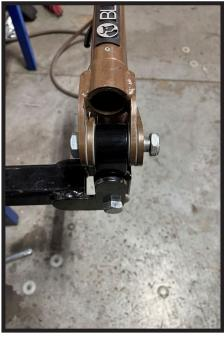
14. Insert 3/4" x 3-1/2" bolt with nut and tighten.
