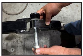
5. Line up the new pivot block with the existing washers and holes in the hitch connector. Start the 3/4" x 3-1/4" bolt. Then insert the other two (2) existing washers on the other side of the pivot block. Fully install bolt with nut and tighten.
