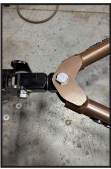
13. Bring tow bar legs back to a horizontal position and remove bolt. Use alignment tool to ensure all holes are aligned.
