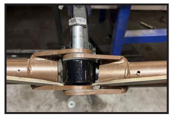
11. Using a rubber mallet, tap end of bolt up far enough to insert the washer.
