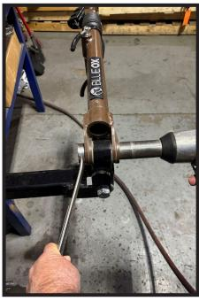
Place tow bar in a stored position. Using a 1-1/8" socket and wrench, remove the one (1) 3/4" nut attaching the tow bar legs.
