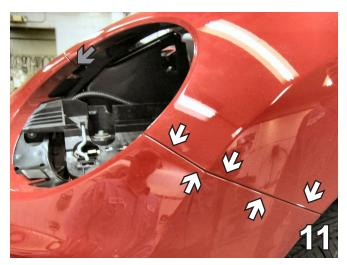
11. Using a T30 Torx socket, remove five metric bolts found in the area where the fascia and the front fender join, as indicated by the white arrows in the photo above. Two plates are also removed when the bolts are removed. Do this to both sides of the vehicle. Set bolts and plates aside to reinstall later.
