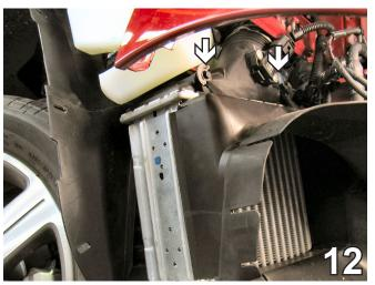
12. Lift the fascia up, disconnect marker lights and temperature sensor (if the vehicle is equipped with such features). Use a 1" x 4" x 22" block of wood (not provided) as a brace to prop up the fascia. Remove the air dam shield immediately in front of the turbo cooler (if equipped on vehicle) simply by pulling it forward. Doing this releases it from two clips. Set air dam shield aside to reinstall later.
