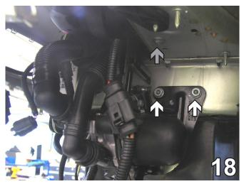
18. Using the 13MM socket, remove two metric bolts from the cooling system bracket (see white arrows). Using the 10MM socket, remove one metric bolt (that secures a support bar) from the frame extension (see grey arrow). Move coolant bracket and support bar out of the way. Do this to drivers side only.
