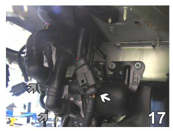
17. On the driver's side, disconnect the electrical connection to the coolant fan (see white arrow). Disconnect the two air lines (see grey arrows) by squeezing the sides of their lower ends to release clips.
