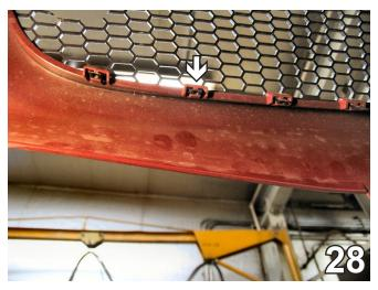
28. Remove the center grille by releasing the 15 clips the clips on the backside of the fascia. Eight on the top edge of the opening and seven on the bottom edge of the opening. The photo above shows several of the clips for illustration. Pull the center grille forward to remove and set aside to reinstall later.
