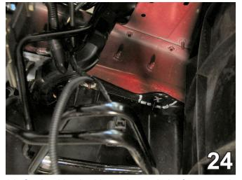
24. On the driver's side, underneath the frame, mark and trim a large enough area to gain access to a hole in the bottom frame that will be used for inserting nut plates later. Do this to both sides of the vehicle. Driver's side is shown. If the vehicle is equipped with a turbo cooler (on the passenger's side), find a dimpled section of plastic to mark and trim around - found between the turbo cooler and the frame, in the same location on the driver's side.
