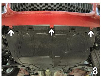
8. Use a small flat screwdriver to remove three push pins on the lower side of the fascia. See next step for removal technique.
