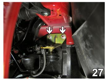
27. Reinstall horn bracket and metal bumper.
