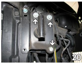
20. Using a 13MM socket, remove the three bolts from the bumper bracket on the driver's side. On the passenger side remove the top two bolts. There is no bolt in the bottom hole.
