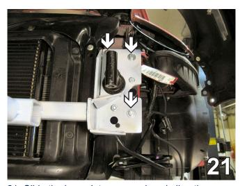
21. Slide the baseplate over and encircling the bumper bracket. Align the baseplate with the three existing holes of the bumper bracket (white arrows). Insert the 8MM-1.25 x 30MM hex bolts and fasten to the 5/16" lock washers and 5/16" flat washers to these bolt locations. Do this to both sides of the vehicle. Baseplate painted white to enhance visibility.
