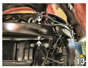
13. Remove the metric hex nut on the bottom of the metal bumper, using the 18MM socket and wrench, remove the metric bolt. Do this to both sides of the metal bumper. Remove metal bumper by pulling forward. Set bolts, hex nuts and bumper aside to be reinstalled later.
