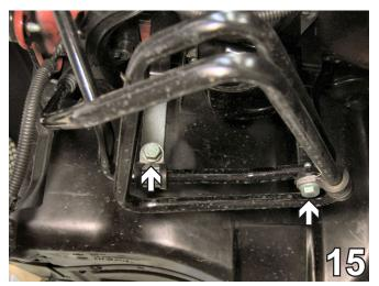
15. Just below the horn bracket, use a 13MM socket to remove two metric bolts securing a coil. Pull coolant coil down out of the way. Set bolts aside to reinstall later.
