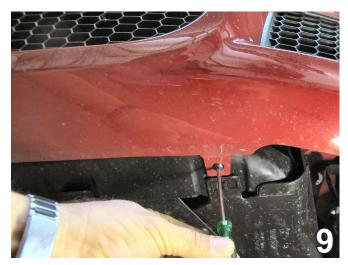
Using the small flat screwdriver, push up on the center of pushpin. The pushpin is released. Do NOT push center push pin all the way through the base. Pry the pushpin out with the screwdriver. Set push pins aside to reinstall later.
