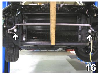
16. Note: Only perform steps 16-18 for vehicles that have the type of coolant system shown in photos. Using the 13MM socket, remove two metric bolts at each end of the coolant line. Set bolts aside to be reinstalled later. Move coolant line out of the way.
