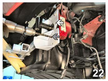
22. Using the baseplate as a template, drill two holes into the frame end using a 13/32" drill bit. From the backside of the baseplate, insert a 3/8-16 x 1 ¼" hex bolt and fasten to the 3/8" lock washer and 3/8-16 hex nut (grey arrow). From the front side of baseplate, insert a 3/8-16 x 1 ¼" hex bolt and fasten to the 3/8" lock washer and 3/8-16 hex nut (white arrow). Do this to both sides of the vehicle.
