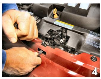
4. Insert and twist a flat screwdriver to separate the hood release handle from the pins securing it.
