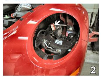
2. On the driver's side, push down on a silver clip found behind the battery box and headlight housing. It can only be reached from above, so a long tool such as a screwdriver is needed to reach it. With the clip pressed down, pull headlight assembly forward to remove. A firm tug may be needed to release the headlight assembly from the electrical plug (see the white arrow in the photo above). Do this to both sides of the vehicle. Set headlight assemblies aside to reinstall later.
