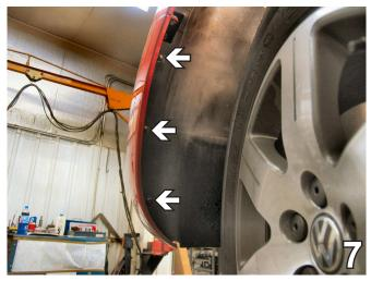
7. Inside the wheel well, just forward of the front tire, use a 25 Torx socket to remove three screws. Set screws aside to reinstall later. Do this to both sides of the vehicle.
