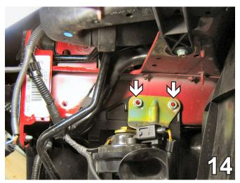
14. Using a 13MM socket, remove two hex nuts securing the horn bracket to the frame rail on the driver's side. Disconnect the horn. Set horn bracket and bolts aside to reinstall later.
