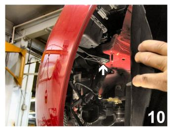
10. On the driver's side, pull the wheel well cover back. Use a 10MM socket to remove the hex nut from the air baffle. Pull down on the air baffle and swivel out of the way for easier access to the metric bolts to be removed later. This is only done to the driver's side. Set bolts aside to reinstall later.
