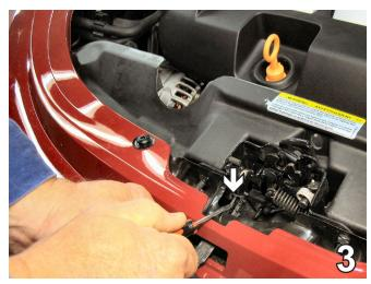
3. Start the removal of the hood release by moving its clip upward. The hood release will move slightly up. A cloth placed under the screwdriver may reduce contact with painted surface and protect the finish.
