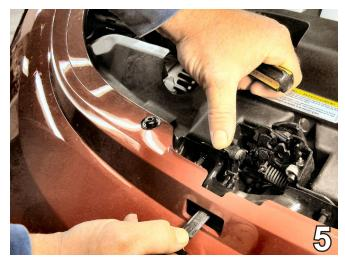
Move hood release handle upwards and carefully guide the hood release out. Pay special attention to not allow the clip to fall out while guiding the hood release out. Set hood release handle aside to reinstall later.
