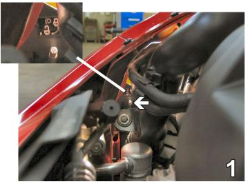
Locate a hex-head pin on the passenger's side, above the bottom of the headlight housing. Near it is a decal with a lock/unlock symbol. Loosen (unlock) the pin by rotating it clockwise. Pull the headlight assembly forward slightly. Do this to both sides of the vehicle.
