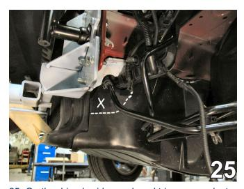
25. On the driver's side, mark and trim an area just below the wiring harness. Doing this allows the wiring harness to be moved while drilling. Avoid cutting the wire harness when using the utility knife.
