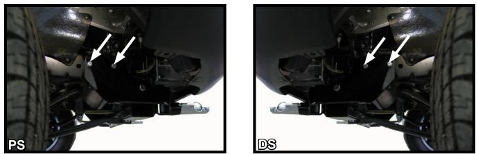
8. Insert 3/8"-16 x 2" bolts with 3/8" lock washers into the holes from the outside of the frame.
