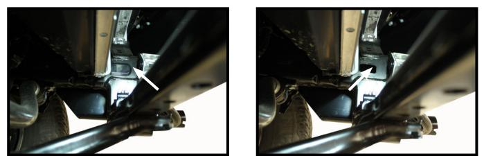
9. On the inside of the frame, remove the cap on BOTH sides of the vehicle. Install 3/8-16 nut plates onto the 3/8" x 2" bolts from step #8. Fully tighten all bolts and reinstall the caps.
