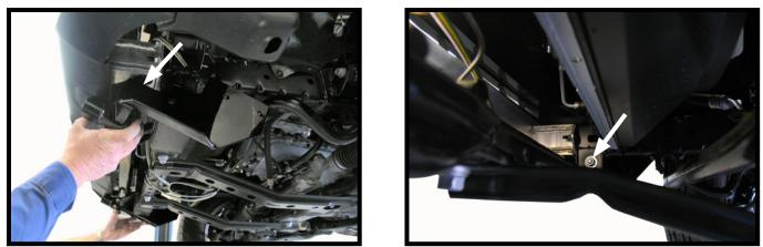
6. Tilt the back of the baseplate down, slide cross tube between the tie down loops and the tab. Align the forward hole of the baseplate with the existing hole of the lower extension that has the 7/8" O.D. spacer tube inserted. Place the 1/2" x 4" hex bolts through the outside of the baseplate and hand tighten.
