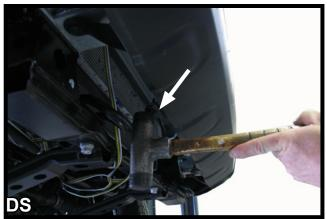
4. Remove the two (2) push pins from the bottom edge of the front fascia. After removing the push pins, use a rubber mallet to bend the tabs upward where the push pins were located.
