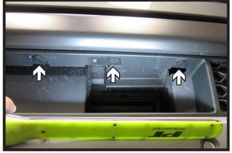
3. Remove the five (5) push pins from the top of the grille opening.
