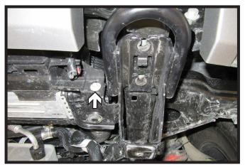
Using an 8MM socket, remove the one
