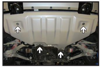
Using a 15MM socket, remove the four
