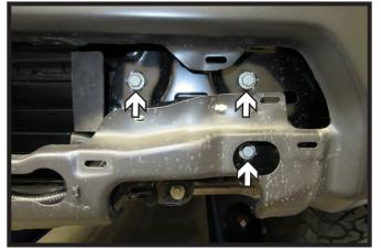
Using a 15MM socket, remove the three (3) bolts from the bumper bracket. Do this on both sides of the vehicle.
