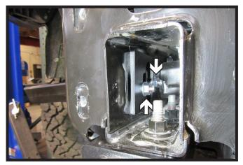
15. Install 3/8" bolts with flat washers into side baseplate holes (left). Install spacer plate with lock nuts on the inside of the frame (right). Ensure the spacer plate is centered on the inside of the frame. Do this on both sides of the vehicle.
