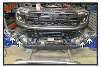
Disconnect the two (2) electrical connections on each side of the bumper. Unclip the rest of the wire loom from the back of the bumper.
