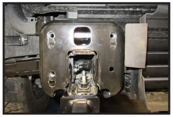
16. Loosen the nut on the back side of the bumper bracket (left). Slide bracket upward so the holes are at the top of the slots on the bracket as shown (right). Retighten nut. Do this on both sides of the vehicle.
