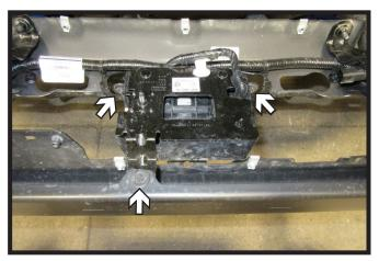
Using a 10MM socket, remove the three
