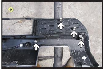
6. Release the eight (8) clips, four (4) on each side from the back of the fascia. As the fascia is removed, disconnect the electrical connection on the driver side of the vehicle. Remove fascia and set aside to be reinstalled later.
