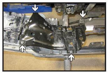
Unclip the wire loom from the metal shield on the backside of the bumper. Then using a T40 Torx, remove the four (4) bolts attaching the shield to the bumper. Remove shield and set aside to be reinstalled later. Do this on both sides of the vehicle.
