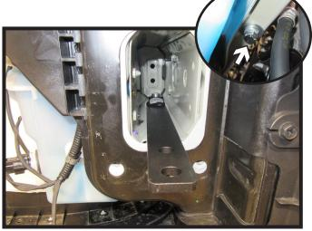
9. Insert frame support bracket as shown. Start the one (1) 5/8" bolt from the bottom of the frame with hardware (inset). Do this on both side of the vehicle.
