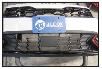
17. Using a reciprocating saw, trim the fascia as shown to allow clearance for the attachment tabs and convenience links.
