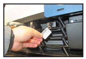
18. Optional: If attaching a breakaway switch, remove the white tag from the pin so that it does not interfere with the ACC.
