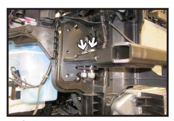
10. Slide the baseplate into place. Insert the two (2) 1/2" bolts with hardware into the baseplate lining up the baseplate and support bracket holes. Leave loose. Do this on both sides of the vehicle.
