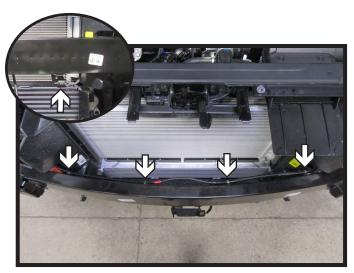
Unsnap the wire loom from the back of the bumper. Remove temperature sensor from bracket (inset). Let hang, it will be repositioned later.
