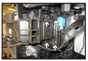
7. Using a 12MM socket, remove the four (4) bolts (white) from the bumper. Then using a 10MM socket, remove the one (1) nut (gray). Do this on both sides of the vehicle. Remove bumper and set aside, it will not be reinstalled.
