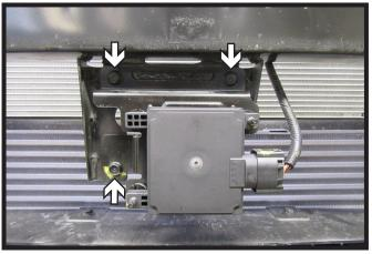
Using a 10MM socket, remove the three
