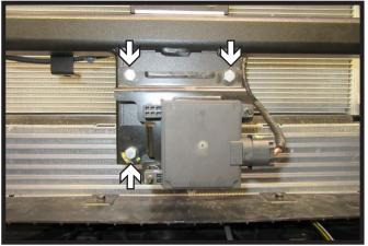
15. Attach the ACC to the bracket on the baseplate using three (3) 1/4" x 3/4" bolts with nylon lock nuts.
