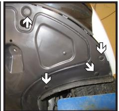
3. Remove the ten (10) push pins from the underside of the fascia, there are four (4) on each side and two (2) in the middle.
