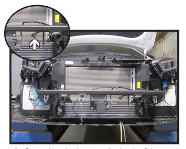
16. Snap the wire loom to the back of the baseplate using original clips. Using the provided zip tie attach the temperature sensor to the baseplate on the driver side of the vehicle letting it hang just below the baseplate (inset).
