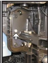
13. Using a 3/8" drill bit, drill the one (1) hole as indicated. Install the 3/8" bolt with hardware. Do this on both sides of the vehicle.
