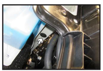
8. Remove the plastic plug from the bottom of the frame in front of the tire. Do this on both sides of the vehicle.
