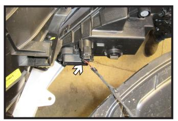
4. As the fascia is removed, unplug the electrical connection on each side. Set fascia aside to be reinstalled later.
