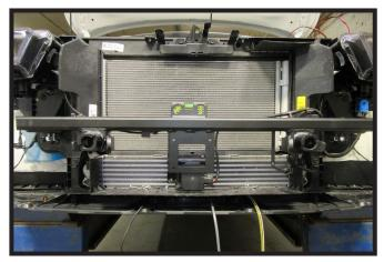
12. Ensure the baseplate is level then tighten all bolts at this time starting with the 8MM bolts. Do this on both sides of the vehicle.
