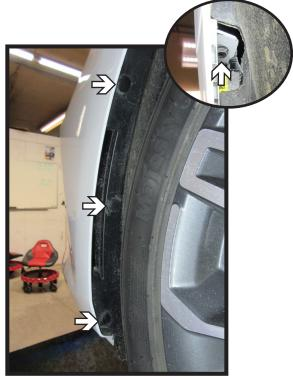
2. Remove the three (3) push pins from along the edge of the wheel well. Then using an 8MM socket remove the one (1) bolt from the fascia joint (inset). Do this on both sides of the vehicle.
