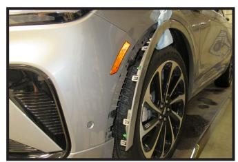
3. Pull back the wheel well trim past the fascia joint releasing the clips. Hold in place with a soft cloth. Do this on both sides of the vehicle.
