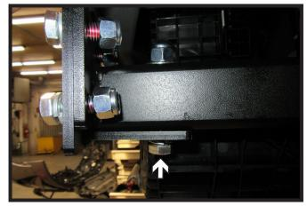
20. Start the one (1) 1/2" bolt in the bottom hole of the center piece with lock washer, flat washer, and nylon lock nut. Leave loose. Do this on both sides of the vehicle. Note: May need to ream out hole with a 1/2" drill bit.
