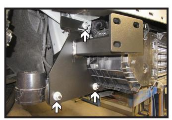
14. Slide the passenger side baseplate piece onto the vehicle and start the three (3) existing nuts. Leave loose at this time.
