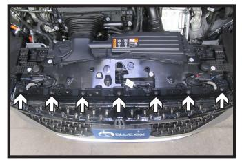
Using a 10MM socket, remove the seven(7) bolts from the top of the fascia.
