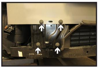
10. Using a 13MM socket, remove the four (4) bolts attaching the support bracket to the bottom and top bumper. Remove bracket, it will not be reinstalled. Do this on both sides of the vehicle.
