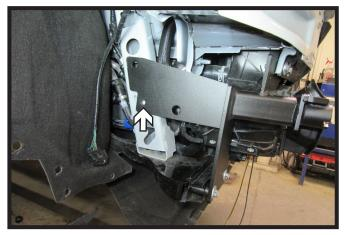
Using a 3/8" drill bit, drill out bottom hole on the side of the vehicle using the baseplate as a template. Do this on both sides of the vehicle.
