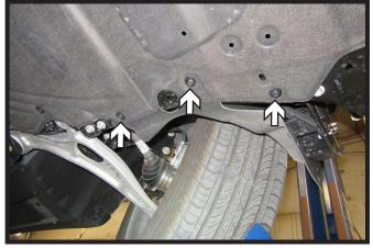
9. Using a T30 Torx, remove the three (3) bolts from the belly pan next to the tire. Do this on both sides of the vehicle. Let belly pan hang.
