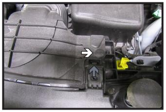
2. Remove the one (1) push pin (white) from the top of the fascia. Then push down on the hook (gray) to release. Do this on both sides of the vehicle.
