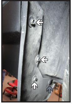
5. Using a 7MM socket, remove the three (3) bolts (white) and one (1) push pin (gray) in front of the tire. Do this on both sides of the vehicle.
