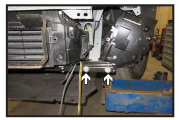
12. Using a 13MM socket, remove the two (2) bolts from driver side of the vehicle.
