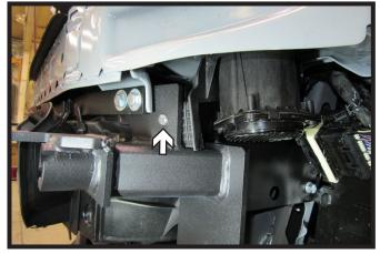
20. Reinstall speaker on the driver side of the vehicle to baseplate using one (1) 1/4" bolt with nylon lock nut.
