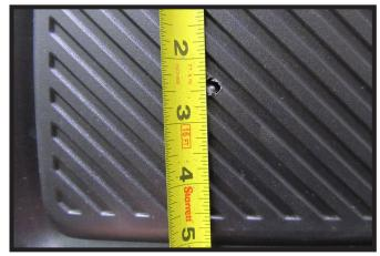
22. Drill small hole into fascia at 3-1/4" across and 2-1/2" down. Start with a small drill bit and move to a larger drill bit.
