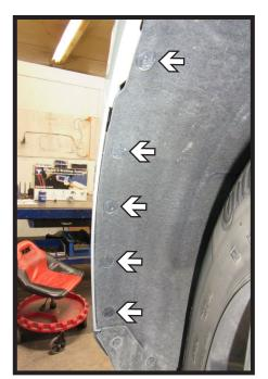
3. Remove the five (5) push pins from along the edge of the wheel well. Do this on both sides of the vehicle.
