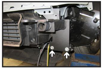
13. Slide baseplate onto driver side of the vehicle and install two (2) existing bolts into bottom hole. Leave loose.
