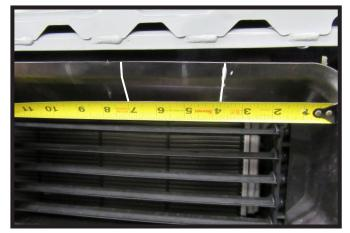
Using a utility knife, trim the top of the shroud on the driver side of the vehicle from 3-3/4" to 7" and then down approximately 2-1/4" as shown.
