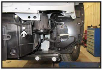
8. Using an 8MM socket, remove the one (1) bolt from the speaker mount on the driver side of the vehicle. Set speaker aside to be reinstalled later.
