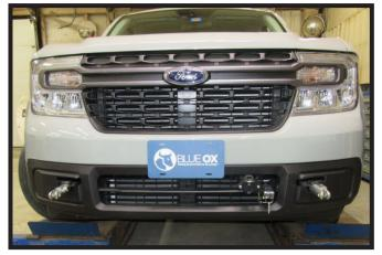
24. Reinstall the belly pan, fascia and reconnect electrical on passenger side of the vehicle.
