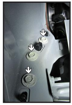
4. Pull back the wheel well liner. Using a 10MM socket, remove the three (3) bolts from the fascia joint. Do this on both sides of the vehicle.
