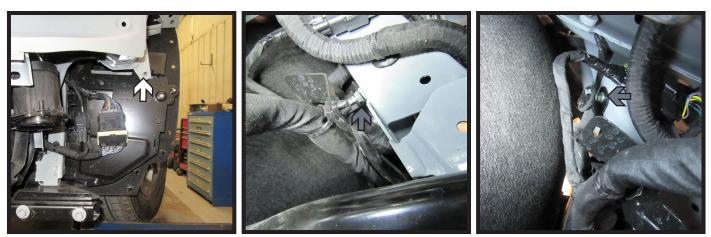
Using a 10MM socket, remove one (1) nut (white) and two (2) bolts (gray) attaching the box to the frame on the driver side of the vehicle. Let box hang. Let box hang.
