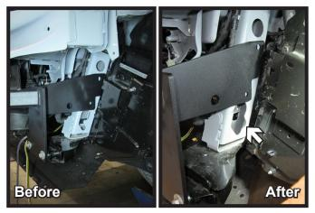
17. Using pliers, bend back the metal piece on the side of the frame creating an access hole for the nut plate. Do this on both sides of the vehicle.
