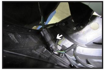
7. Remove fascia and unplug electrical on the passenger side of the vehicle.
