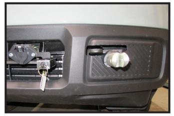
23. Hold the fascia as close to its original position, mark and trim the fascia around the convenience links and attachment tabs using hole as starting point.
