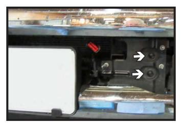
16. Reinstall bumper, insert the existing two(2) bolts into the inside holes on both sides of the vehicle and reconnect the wiring.
