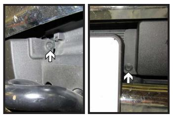
Models with Adaptive Cruise Control (ACC): Using a 10MM socket, remove the two (2) bolts from the cover of the ACC on the driver side of the vehicle.
