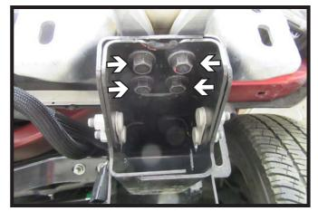
Using an 18MM socket, remove the four
