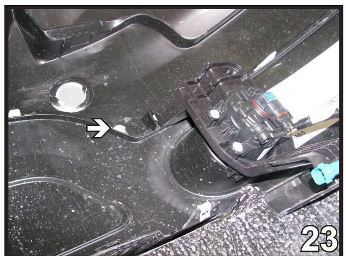
23. On the backside of the fascia by the fog light, cut the white tab off. Do this on both ends of the fascia.
