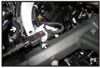
10. Unplug the three (3) electrical connections, one (1) on the driver side and two (2) on the passenger side, from behind the bumper.
