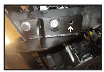
21. Using a 1/2" drill bit, drill out the back bottom hole using the baseplate as a template. Do this on both sides of the vehicle.
