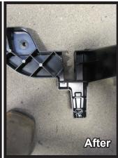
27. Using a reciprocating saw, trim the plastic piece from behind the bumper as shown. Do this on both sides of the piece. Reinstall plastic piece.
