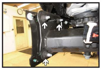
12. Using an 18MM socket, remove the three (3) nuts from the back of the bumper. Do this on both sides of the vehicle. Slide bumper and lower shutter piece off the vehicle and set aside to be reinstalled later.
