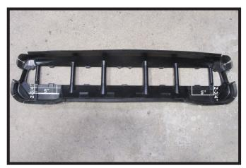
24. Using a reciprocating saw remove the indicated area of the shutter housing to allow clearance for the baseplate and convenience links.
