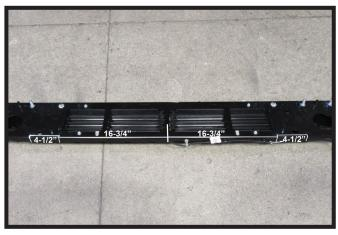
14. Mark the center point on the back of the bumper. Measure 16-3/4" in each direction and mark. Then measure 4-1/2" and mark again.
