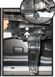
Using a 10MM socket, remove the two
