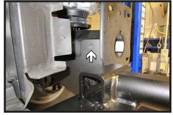
19. Ensure the baseplate is as far back as possible. Using a 1/2" drill bit, drill out the side hole using the baseplate as a template. Do this on both sides of the vehicle.
