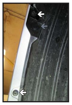
Using a Phillips screw driver remove the two (2) screws (white) from the wheel well. Then remove the one (1) push pin (gray).
