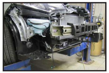
Reinstall the bumper on the vehicle. Then reinstall the windshield washer fluid reservoir to the passenger side of the vehicle.
