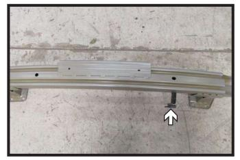
9. Remove the temperature sensor bracket from the bumper. Set aside to be relocated and reinstalled later.
