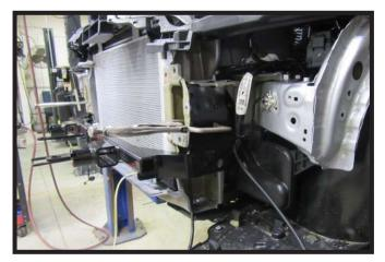
10. Tilt baseplate to slide into place. Make sure that the baseplate is as far upward and forward as possible. Then clamp into place.
