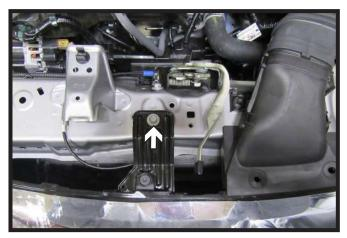
Using a 10MM socket to remove the one (1) bolt.
