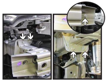
Using a 10MM socket remove the five (5) bolts attaching the bumper to the frame. Do this on both sides of the vehicle. Remove bumper and set aside to be reinstalled later.
