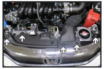
1. Remove the five (5) push pins from the fascia cover. Remove fascia cover and set aside to be reinstalled later.
