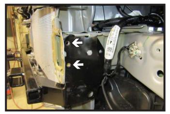
Using a 3/8" drill bit, drill out the front two (2) holes. Do this on both side of the vehicle.
