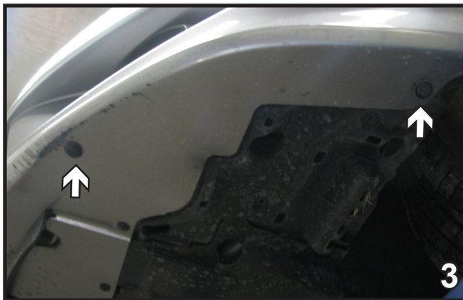
3. Using a flat screwdriver, remove two (2) push pins from the bottom corner of the fascia. Do this to both sides of the vehicle.
