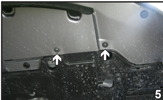
5. Using a Phillips screwdriver, remove two (2) screws holding the fascia. Do this to both sides of the vehicle.
