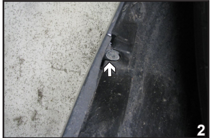
2. Just inside wheel well, on edge of fascia, use the Phillips screwdriver to remove one (1) screw. Do this to both sides of the vehicle. Set screws aside to be reinstalled later.
