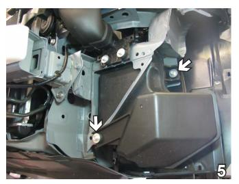
On the driver's side, remove two metric bolts from the air baffle using the 10mm socket. Pull air baffle down and out to the side of vehicle to remove. Set bolts and air baffle aside to be reinstalled later.
