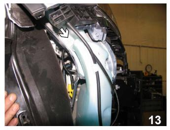
13. **2010 Model:** Remove one metric bolt from the back side of washer reservoir using the 10mm socket. Pull reservoir down and to the side to remove. Set bolts and reservoir aside to be reinstalled later.
