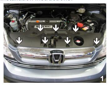
Remove seven pushpins from the top of the radiator cover. Pull radiator cover forward to remove. Set radiator cover and pushpins aside to be reinstalled later.
