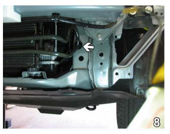
8. On driver's side, remove the coolant line clip from the front of lower frame support just below metal bumper. Do not remove clip from coolant line. Pull the driver's side end of coolant line over to the passenger side of vehicle to clear area for baseplate installation.
