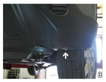
On driver's side, remove one metric bolt from the lower edge of fascia, just forward of front tire, using the 10mm socket. Do this to both sides of vehicle. Set bolts aside to be reinstalled later.
