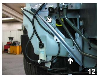
12. On the passenger's side, disconnect and plug the washer reservoir. Remove two metric bolts from the front of reservoir using the 10mm socket. Set bolts aside to be reinstalled later.
