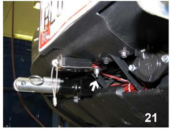
21. Attach the breakaway (not supplied) to the bracket with 1/4"-20 x 3/4" bolt and 1/4"-20 nut.
