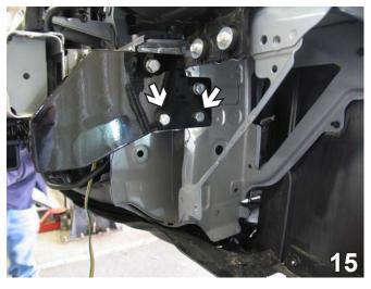
15. In lower drilled holes of baseplate, install two 3/8-16 x 1" hex bolts, 3/8" lock washers and 3/8-16 hex nuts and tighten. Do this to both sides of the vehicle.
