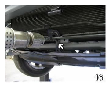
16. Relocate coolant line lower. Move bottom coolant line to just above original bolt hole for the bracket. Drill into the bracket using the 9/32" drill bit. Insert 10mm metric bolt into drilled hole and tighten.
