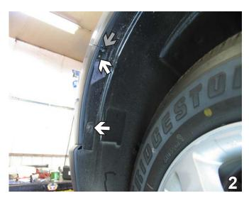
Just forward of front tire, inside the wheel well, remove two Phillips screws (see white arrows). Remove one pushpin on the corner of fascia, just above the upper Phillips screw (see grey arrow). Do this to both sides of the vehicle. Set screws and pushpins aside to be reinstalled later.
