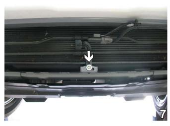
Using the 10mm socket, remove one metric bolt from the coolant line bracket at the bottom of radiator. Set bolt aside to be reinstalled later.
