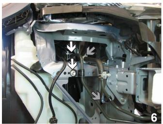
6. On passenger's side, on coolant line closest to washer reservoir, remove one metric bolt using the 10mm socket (see lower white arrow) and disconnect one clip from line (see upper white arrow). On the coolant line closest to frame, disconnect two clips (see grey arrows). The two upper clips will remain on vehicle and the two lower clips are to remain on coolant lines.
