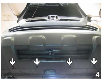
Remove four pushpins from the bottom of fascia. Pull fascia corners to the side, then forward to remove. Set pushpins and fascia aside carefully to be reinstalled later.
