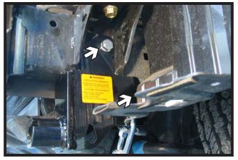
15. Insert the nut plate into the drilled hole on the frame cap to align with the drilled hole, tighten the 1/2"-13 hex bolt and 1/2" lock washer into the drilled hole. Repeat on other side.
