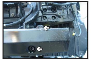
10. Remove the two (2) bolts from the metal bumper with a 17MM socket. Do this on both sides.
