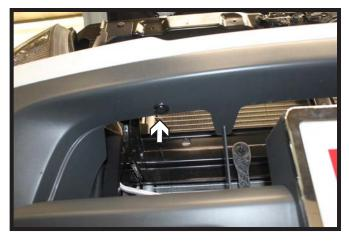
8. On the top side of the lower grille opening remove the three (3) push pins.
