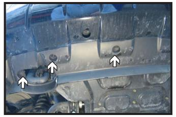
On the underside of the fascia, using a 10MM socket, remove the six (6) screws from the shrouding. There are three (3) on each side. Set the shroud aside.
