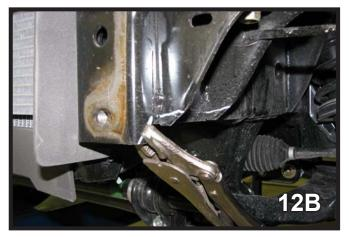
12. Using the vise grip bend the frame support, approximately 1/2" up from the bottom, back and fourth until it snaps off on both the front and back supports. Do this on both sides. (14A) On 2011-12 Models: In addition to front and back supports, snap off the area in front of the supports for additional baseplate clearance. Do this on both sides (14B)
