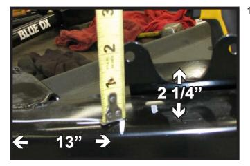
17. Set the metal bumper on a bench, clamp the electrical bracket to the back of the driver's side with the vise grip. The bracket should measure 13" from the driver's end of the metal bumper and 2 1/4" from the top edge of the bumper to the top hole location. Attach the bracket with the two (2) #10-16 self drilling screws using the 5/16" nut driver. Reinstall the metal bumper with the existing bolts.
