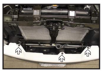
3. Remove three (3) push pins from the top of the fascia.
