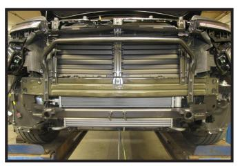
17. Reinstall the impact bar onto the bumper and tighten support bracket bolts. Then reinstall bolts attaching top shutters to bumper.
