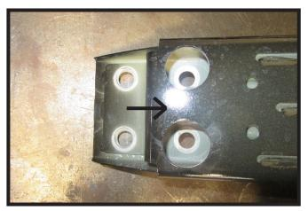
14. If needed, use a reamer to slot the four (4) holes 1/8" to 1/4" on the bumper towards the inside. Do this on both sides of the bumper.
