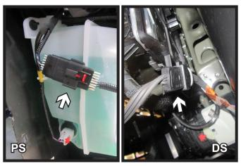
7. As the fascia is removed, disconnect the one (1) electrical connection on the passenger side and the one (1) on the driver side of the vehicle. Set fascia aside to be reinstalled later.
