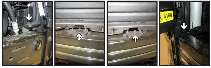
8. Using a 7MM socket, remove the four (4) bolts, one (1) on each side and two (2) along the center, attaching the upper shutters to the bumper.
