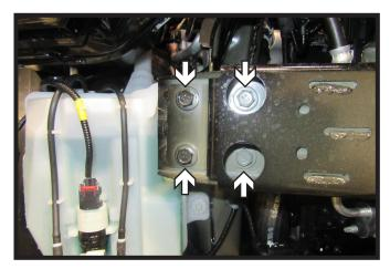
Using a 15MM socket, remove the four (4) bolts from the bumper. Do this on both sides of the bumper. Remove bumper and set aside to be reinstalled later.
