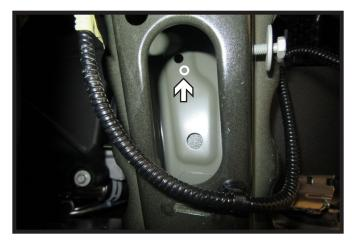
20. Hold the support plate in place as shown on passenger side of the vehicle so the front holes and back bottom hole line up with the existing holes on the vehicle. Mark frame using the baseplate as a template for top back hole. Using a 1/4" drill bit, create starter hole in frame. Then using a 1/2" drill bit, drill out top hole in frame.
