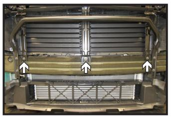
Using a 10MM socket, remove the three
