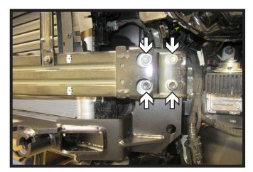
16. Slide the baseplate onto the vehicle between the frame and the bumper. Start one (1) existing 10MM bolt in the top outer hole. Do this on both sides of the vehicle. Level baseplate and ensure the holes on the bumper line up with the baseplate. Install the remaining three (3) existing bolts on each side of the vehicle.
