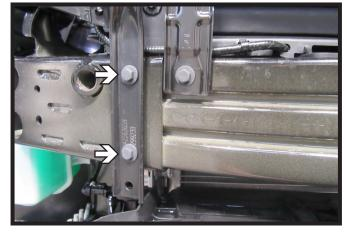
10. Using a 10MM socket, remove the two (2) bolts on each side connecting the impact bar to the bumper. Set bar aside to be reinstalled later.
