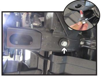
14. Start the bottom 1/2" x 1-3/4" bolt with lock washer, thick washer, and slotted plate. Press baseplate up and in while hand tightening the bolt. Do this on both sides of the vehicle.
