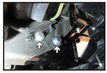
6. Insert two (2) 1/2" bolts with flat washers and spacers. Do this on both sides of the vehicle.
