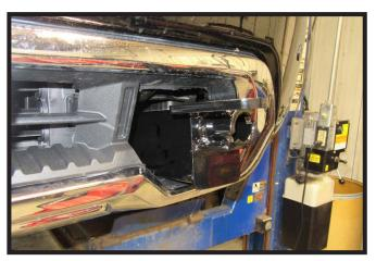
5. Tip the baseplate up slightly and slide it into the tow hook housing. Do this on both sides of the vehicle.
