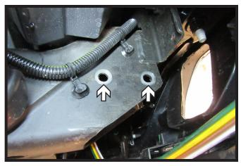
3. Using a 13/16" drill bit, drill out the two (2) holes on the inside of the frame only. Do this on both sides of the vehicle.
