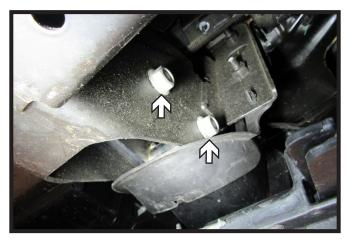
Using an 18MM socket & wrench, remove the two (2) bolts from the tow hook. Remove tow hook, it will not be reinstalled. Do this on both sides of the vehicle.
