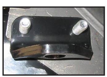
7. Slide the convenience link bracket onto the two (2) 1/2" bolts and place a nylon lock nut on each bolt to secure. Do this on both sides of the vehicle.
