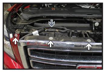
2. Using a 10MM socket, remove the six (6) screws from the top edge of the fascia (white). There are three (3) on each side. On the passenger side, disconnect the wiring harness (gray).
