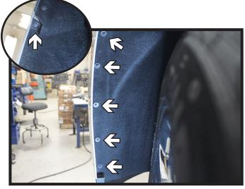
3. Using a 7MM socket, remove the six (6) screws from the edge of the wheel well. Do this on both sides of the vehicle.
