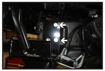
9. Using a 17/32" drill bit, drill out the remaining holes in the inside of the passenger side frame. Install 1/2"-13 x 1-1/2" bolts with lock washers into the hole and a 1/2"-13 whiz nuts on the inside of the frame. Fully tighten all hardware.
