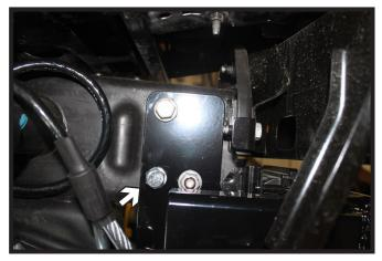
10. On the driver side, install 1/2"-13 x 1-1/2" bolt with lock washer into the hole and a 1/2"-13 whiz nut on the inside of the frame. Fully tighten all hardware.
