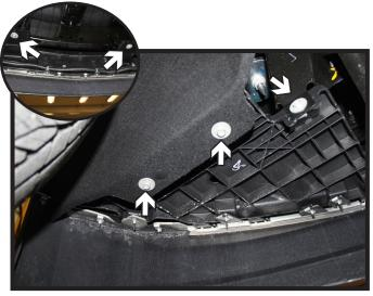
4. Using a 10MM socket, remove the eight (8) screws from the underside of the fascia. There are three (3) on each side and two (2) in the middle.
