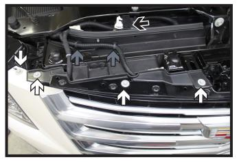
2a. Using a 10MM socket, remove the eight (8) screws from the top edge of the fascia. There are four (4) on each side.
