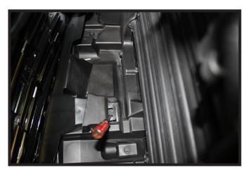
2b. Using a small flat screwdriver, release the two (2) tabs down behind the grille prior to removing the fascia on step 5.
