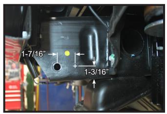
7. Using a 17/32" drill bit, drill a hole thru the frame 1-7/16" back from the existing hole and 1-3/16" up from the bottom of the frame. Do this on the outside DS frame and the inner PS frame. (DS shown)
