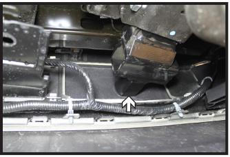
Partially reinstall the fascia with a couple of screws along the top and pull the fascia tight
