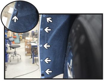
3. Using a 7MM socket, remove the screws from the edge of the wheel well. Do this on both sides of the vehicle. Qty of screws vary per model.
