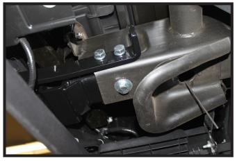
11. Install the convenience link to the frame with 1/2"-13 x 1-3/4" bolts with 1/2" lock washers. Do this on both sides of the vehicle. Tighten down until the frame squeezes against the baseplate.
