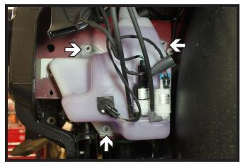
On the driver side, using a 10MM socket, remove the three (3) nuts from the washer fluid reservoir. Disconnect all lines and electrical connections, then set reservoir aside.
