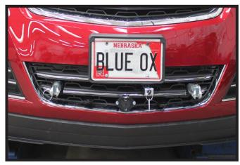
15. Hold the fascia as close to its original position, mark and trim the fascia around the convenience links and attachment tabs. Reinstall the fascia and fascia shroud.
