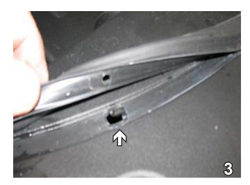
3. Remove the rubber piece across the top by pulling it to unhook it. Push hard on both sides to release the christmas tree clip.
