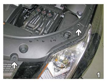
Remove the two (2) push pins on each side from the top edge of the fascia. Do this to both sides of the vehicle.
