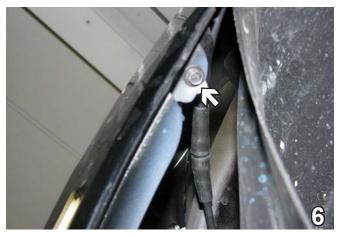
6. Pull the wheel well cover back, using a 7MM socket remove one (1) bolt from the inside corner of the fascia. Do this to both sides of the vehicle.
