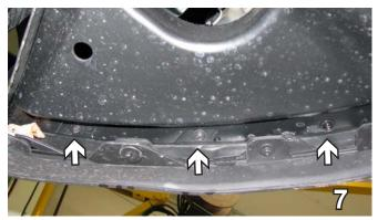
Using a 7MM socket, remove twelve (12) bolts across the bottom of the belly pan.
