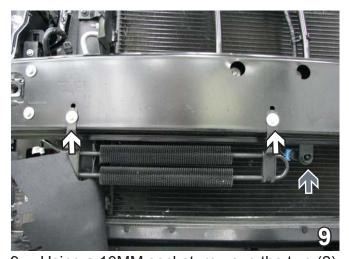
Using a 10MM socket, remove the two (2) bolts and the coolant line.
