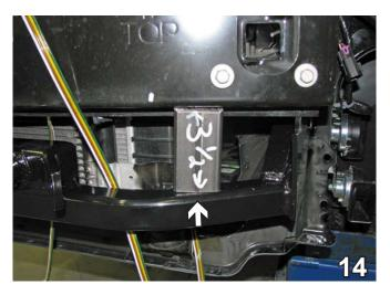
14. Position the baseplate onto the vehicle. Leaving a 3-1/2" gap from the bottom of the bumper to the top of the crosstube of the baseplate. Level and securely clamp the baseplate to the frame.
