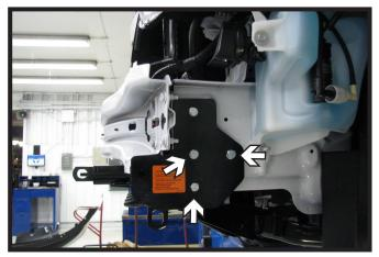
13. Using a 13/32" drill bit, drill the remaining holes thru the frame. Install the 3/8"-16 hardware into the holes with 3/8" nut plates inside of the frame. Do this on both sides of the vehicle. Fully tighten all hardware.
