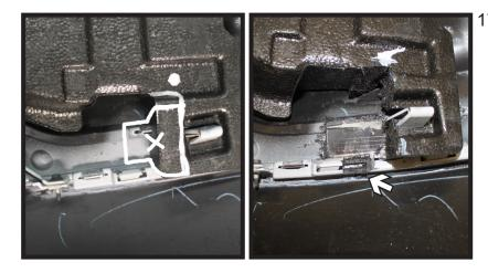
17. **2016 Terrain:** Trim off the end of the styrofoam support and thru the first layer of the fascia in the area as shown (left).
