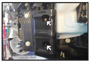
6. **2014-16 Models:** On the driver side, using a 10MM socket, remove the two (2) interior bolts (white) from the reinforcement. Using a 15MM socket, remove the two (2) outer bolts (gray). The reinforcement will not be reinstalled.
