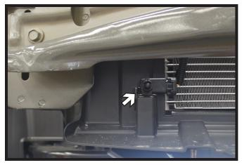
10. Unsnap the temperature sensor and move it aside for baseplate installation.
