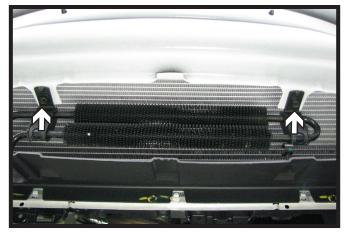
9. If equipped, remove the two (2) bolts from the cooler and move it down to allow the baseplate to be installed.
