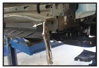
8. Bend the outer flanges of the bumper out approximately 90° to the bottom of the bumper. Do this on both sides of the vehicle.
