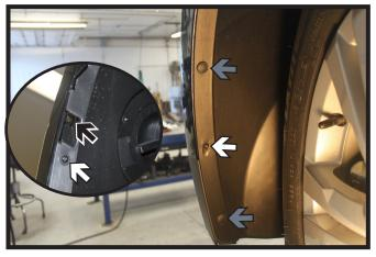
All Models: Using a T20 Torx, remove the two (2) screws from edge of the wheel well (white). Then remove the two (2) push pins (gray).
