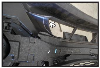
17. **2015-16 Equinox:** Trim off the end of the styrofoam support above the opening (left). On the end of the opening, trim along the seam as shown (right).
