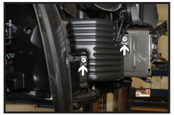
Using a 10MM socket, remove the two (2) nuts from the baffle on the passenger side.
