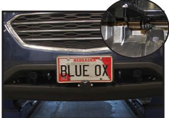
19. Secure the temperature sensor in the desired location (inset). Reinstall the fascia.
