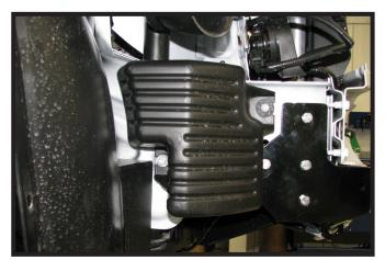
14. Reinstall the air baffle. Putting three (3) washers behind the air baffle on each stud to space the air baffle out from the frame.
