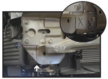
7. Using a reciprocating saw, trim the face of the frame flush with the outside of the frame rail (white) and up to the bumper seam (gray). Do this on both sides of the vehicle.
