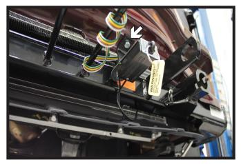
16. Optional: Using a 9/32" drill bit, drill a hole into the bottom side of the bumper centered between the electrical rod and the convenience link. Attach the bracket with 1/4"-20 x 3/4" bolt and 1/4"-20 nut (white). Fasten the breakaway to the bracket with a 1/4"-20 x 3/4" bolt and 1/4"-20 nut.
