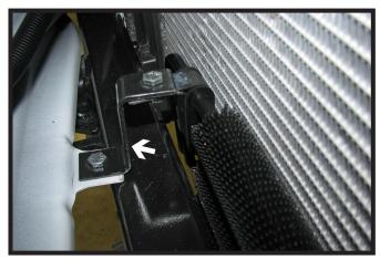
If equipped, reinstall the cooler to the existing tabs with the supplied brackets and 1/4" hardware in between the baseplate and radiator.
