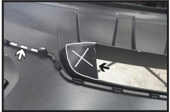
17. **2014 Equinox:** Trim off the end of the styrofoam support above the opening (left). On the end of the opening, trim along the seam as shown (right-black). Then as needed trim off the material between the tabs as needed to clear the baseplate (right-white).
