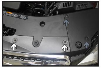
Using a T20 Torx, remove the two (2) screws from the top edge of the fascia (white). Then remove the two (2) push pins (gray). Do this on both sides of the vehicle.
