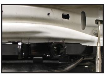
12. Slide the baseplate onto the frame until it is 1-1/8" from the baseplate to the top of the frame (inset). Level and clamp the baseplate securely. Using a 13/32" drill bit, drill the bottom hole in the baseplate thru the frame. Install a 3/8"-16 x 1-1/2" bolt into the hole and install a 3/8" lock washer and lock nut on the inside of the frame. Do this on both sides of the vehicle. Recheck the baseplate is level and fully tighten all hardware.
