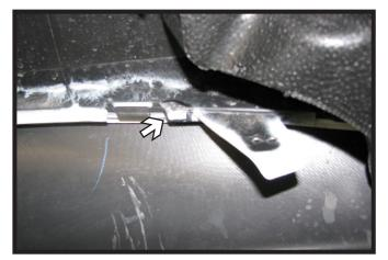
17. **2010-15 Terrain:** Trim off the corner next to the flap to allow for baseplate clearance. Do this on both sides of the fascia.
