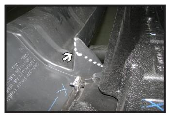
17. **2010-13 Equinox:** Trim the ends of the opening approximately 1" down on the bottom then tapered back to top.
