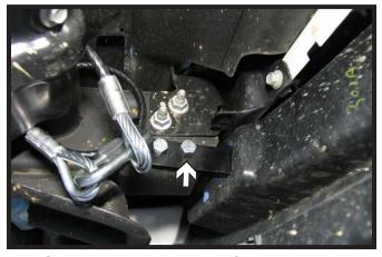
8. Slide the baseplate into frame end to align with the front tow hook hole on the outside of the frame rail. Insert straight portion of the convenience link thru the tow hook opening and align it with the existing holes of the frame. Insert a 1/2"-13 x 5" bolt thru the frame with a 1/2" lock washer and 1/2" lock nut on the other side and tighten down. Do this to both sides of the vehicle.
