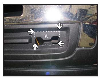
Using a utility knife, trim the top part of the tow hook shield. Do this to both sides of the vehicle.
