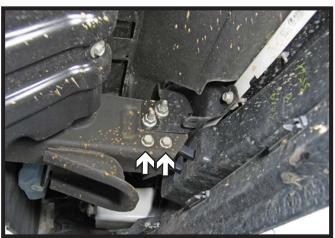
Using a 18MM socket, remove two (2) bolts from the inside edge of the frame rail. Do this to both sides of the vehicle. This hardware will not be reinstalled.
