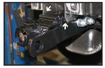
9. Using the existing back hole and the baseplate as a template, drill thru the the frame with a 17/32" drill bit. Insert a 1/2"-13 x 5" bolt into the hole with a 1/2" lock washer and 1/2"-13 nylon lock nut on the back side and tighten down (left).
