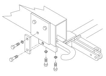
4. Take the flat braces (Items 2 & 3) and fasten them to each side of the frame and to the side of the baseplate. Use the  $1/2 \times 1 3/4$ " bolts, lock washers and nuts (Items 4,5,6) to fasten the brace to the baseplate. Use the existing 14mm bolt to fasten the brace to the frame of the vehicle. Be sure to use Loctite with each bolt. Once all bolts have been started, tighten according to the torque chart in the General Instruction Sheet.
