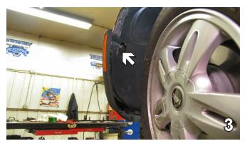
Locate opening in wheel well just forward of front tire, remove two metric bolts with the 8MM socket, on both sides.
