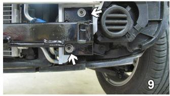
Align holes of baseplate with studs just below metal bumper and reinstall four existing nuts.
