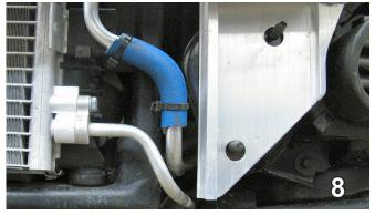
Using a utility knife, make a slit the length on blue 3/8" tubing, wrap the tubing onto driver's side upper coolant line as shown. Secure the tubing to the line with zip ties. This will protect coolant line from rubbing against the back of baseplate.
