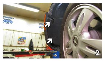
2. Just forward of front tire, on wheel well, are two Phillips head push pins to remove, on both sides.
