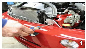
1. Using the T30 Torx, remove the bolts from the top side of fascia.
