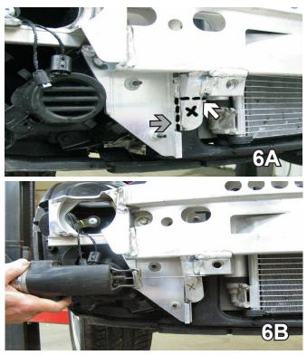
6. Locate tow plate bracket on passenger's side of front bumper. Mark and remove lower gusset just below tow plate bracket with the reciprocating saw, as shown in photos above. This will open area to allow baseplate installation.
