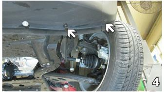
4. Remove the two Phillips screws from the lower edge of front fascia, on both sides.
