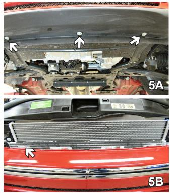
5. Remove three metric bolts from the lower edge of front fascia with the 10MM Socket. Release the four clips on the top edge of fascia, pull fascia forward, unplug all electrical connections and set fascia aside carefully.
