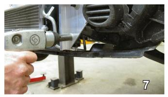
7. Remove the two metric hex nuts just below metal bumper with the 13MM socket, on both sides.
