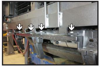
Attach plastic piece from bumper to cross member using four (4) 1/4" x 1" bolts with flat washers and lock washers.
