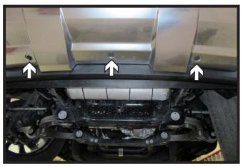
4. Using a 10MM socket, remove the three (3) bolts from the bottom of the fascia.
