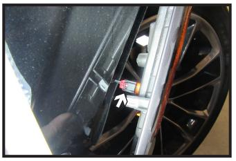
2. Unsnap the wheel well trim past the fascia joint. Unplug light as trim is pulled back. Place soft cloth between trim and vehicle to hold trim out of the way. Do this on both sides of the vehicle.
