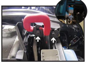
6. Using a 16MM socket, remove the two (2) bolts (white) from the underside of the tow hook. Using a 30MM socket, remove the nut (gray) from the backside of the tow hook (inset). Do this on both sides of the vehicle. Remove tow hooks and set aside, they will not be reinstalled.
