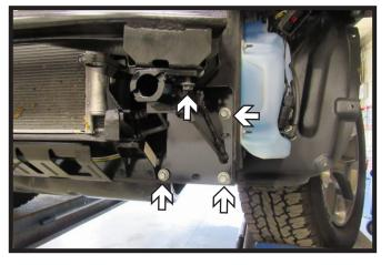
8. Slide the baseplate into place and install the four (4) existing 10MM bolts. Tighten the bumper bolt first, then tighten the remaining three (3) bolts. Do this on both sides of the vehicle.
