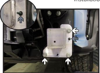
7. Using a 15MM socket, remove the three (3) bolts from the frame extension. Using a 10MM socket, remove the nut (gray) from the frame extension. Do this on both sides of the vehicle. Remove frame extension, it will not be reinstalled. Note: Some models my have a clip that needs to be removed instead of a nut (inset).
