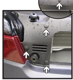
1. Remove the thirteen (13) push pins from the top edge of the fascia cover. There are six (6) on each side and one (1) in the center. Remove fascia cover and set aside to be reinstalled later.
