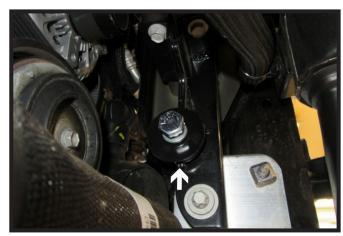
9. From the backside install the 1/2" x 5" bolt with lock washer and 1/4" x 2" DIA washer. Do this on both sides of the vehicle.
