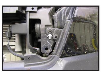
Using a T27 Torx, remover the one (1) screw from behind the fascia cover. Do this on both sides of the vehicle.
