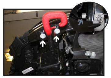
6. Using a 16MM socket, remove the two (2) bolts from the underside of the tow hook (white). Using a 30MM socket, remove the nut from the backside of the tow hook and remove from the vehicle (inset). Do this on both sides of the vehicle.
