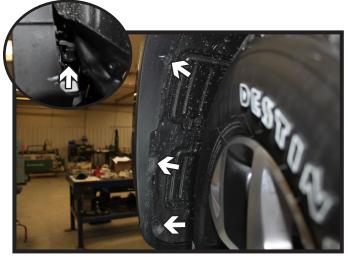
Using a 8MM socket, remove the three (3) screws from the edge of the wheel well. Pull back the wheel well cover, using a 10MM socket, remove the screw behind the trim (inset). Do this on both sides of the vehicle.
