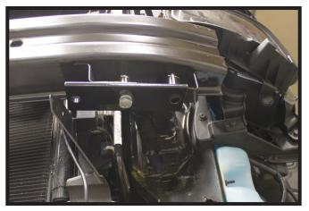
Loosely bolt the bumper attachment plate to the underside of the bumper with the 10MM hardware. Only install Loctite onto the inner bolt (white) and fully tighten. Once the inner bolt is tightened, remove the outer bolt (gray) until the baseplate is installed. Do this on both sides of the vehicle.
