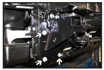
10. Install the baseplate to the vehicle using the three (3) existing extension bolts (white). Install 10MM-1.25 x 40MM bolts with 3/8" flat washers and 10MM lock washers into the lower bumper bolts (gray). Fully tighten all fasteners. Do this on both sides of the vehicle.
