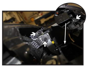
Using a 10MM socket, remove the three
